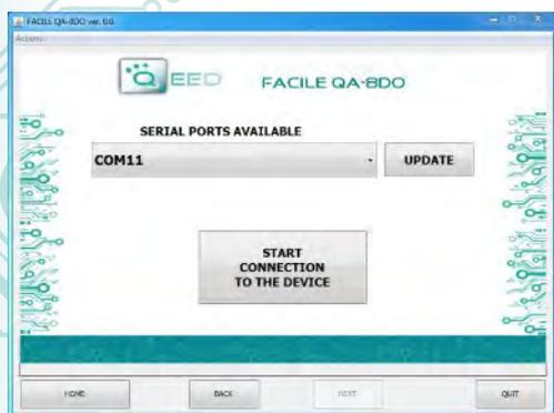
It is possible to use the program without connecting to the module, in this mode you can SAVE the configuration on your PC, which can then be sent to the QA-8DO at a later time.
